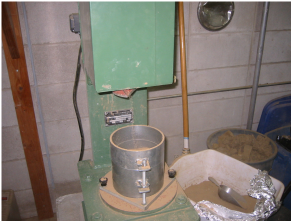
(27k,27l) Dry soil – zero percent moisture, compacted in 6” mold and planed (spilled soil)
