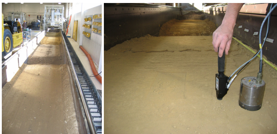
(26a) Trench prepared for testing; (26b) Microwave sensor on air dry compacted soil bed
