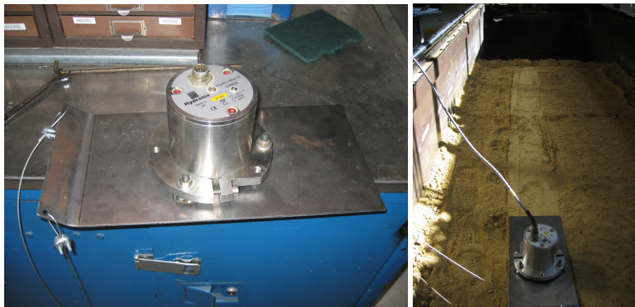
(26e) Sensor placed on steel plate; (26f) Sensor: hand-pulled across the bed
