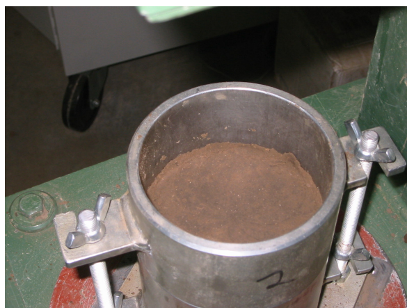
(27h) Compacted sample
