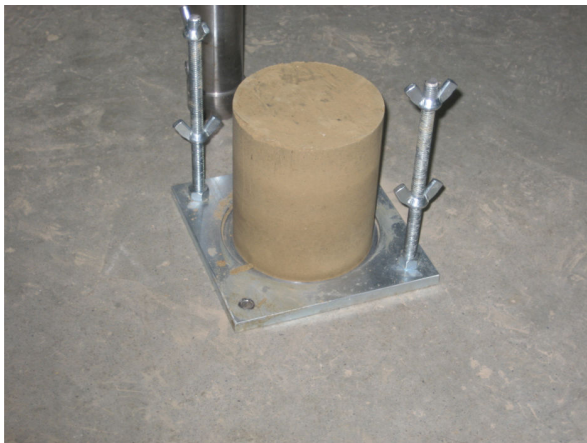
(79i) Sample extraction (79j) Extracted sample resting on top, placed on the ground
