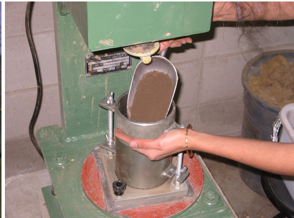
(27f) Placing in the mold in layers
