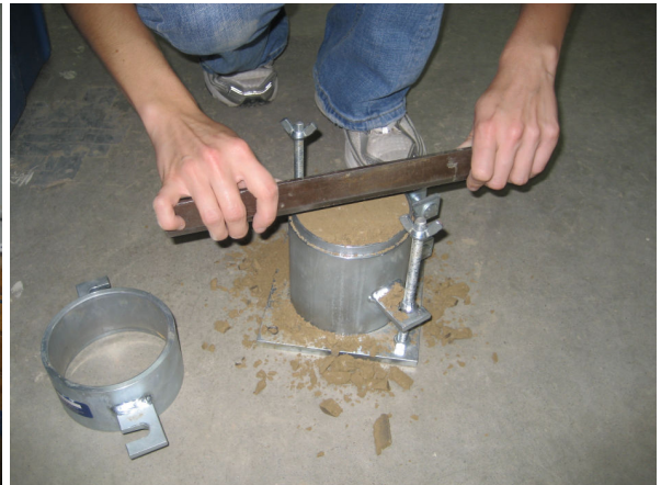
(79e) Compaction in a 4" split mold (79f) Planing the top after compaction
