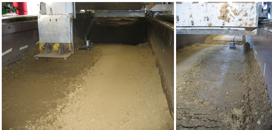
(26q, 26r) Sensor: Machine pulled along the wet side of the soil bed
