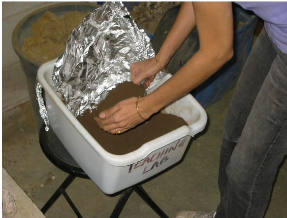
(27e) Mixing soil uniformly just before testing
