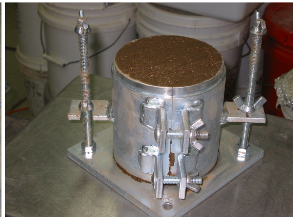
(27n) Wet soil - oozing water at the side of the mold
