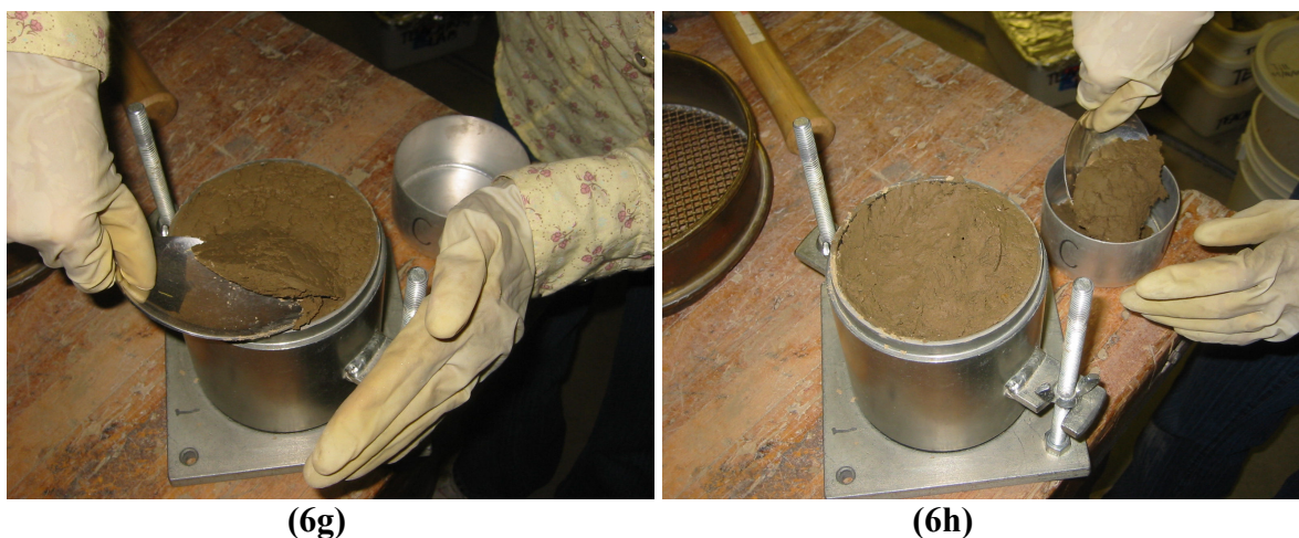
Figures 6(a-h): Microwave sensor testing in lab (sample in the mold)
