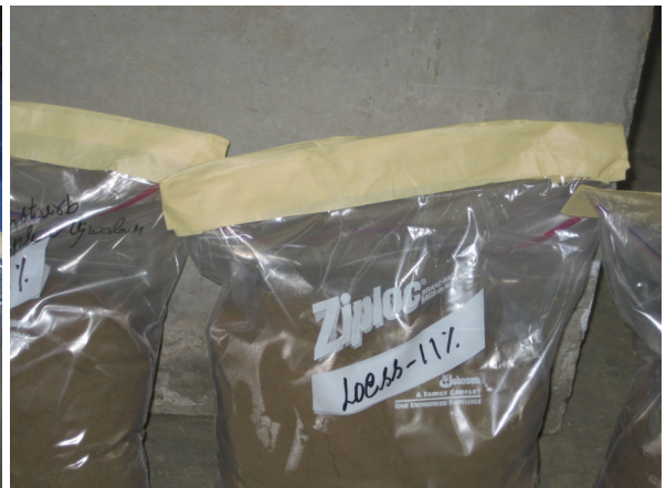
(79c, 79d) Samples packed in plastic bags after mixing required moisture and left for mellowing
