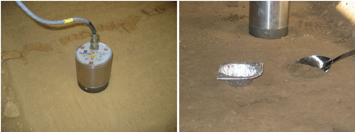
(26c) Sensor on air dry bed; (26d) Sample collection for oven dry test
