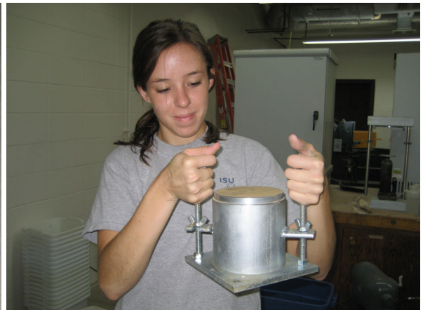
(79g) Planing the top of the sample (79h) Mold surface cleaned and dry density determined
