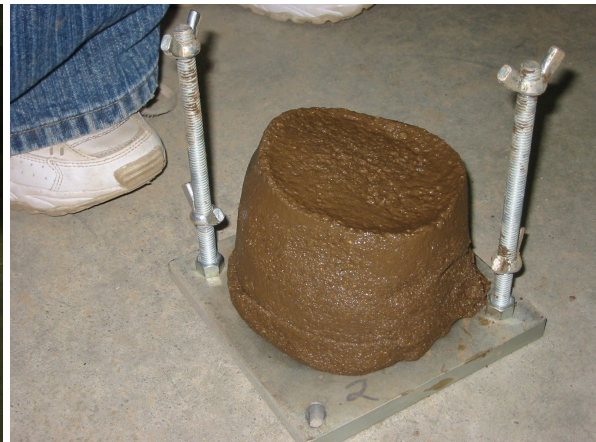
(27r) Very wet sample – collapsed on extraction
