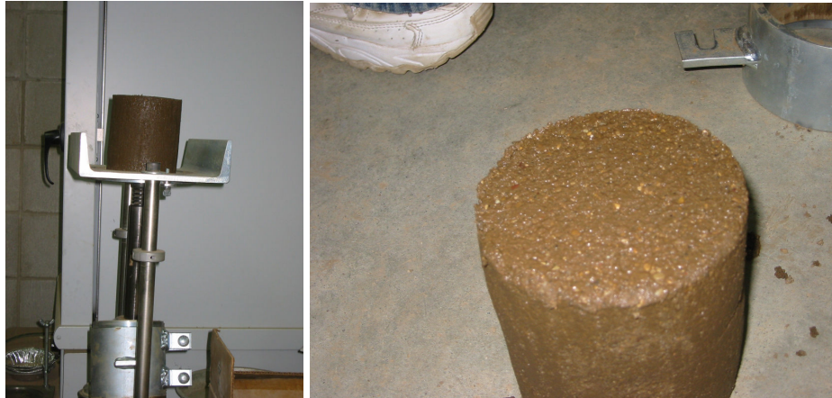
(27o, 27p) Wet sample extracted- moisture can be seen clearly on the surface and sides
