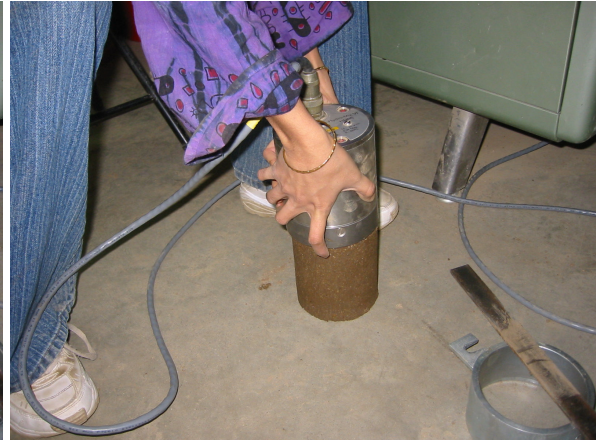
(27j) Sensor placement on the soil sample
