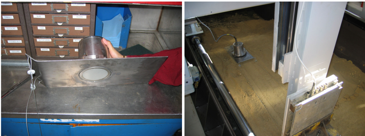
(26g) Sensor base cleaned before testing; (26h) Sensor: Tied to a sled
