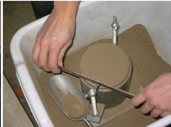
(27k,27l) Dry soil – zero percent moisture, compacted in 6” mold and planed (spilled soil)
