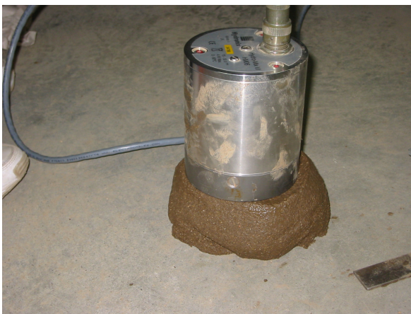
(27s) Sensor testing at very high moisture content
