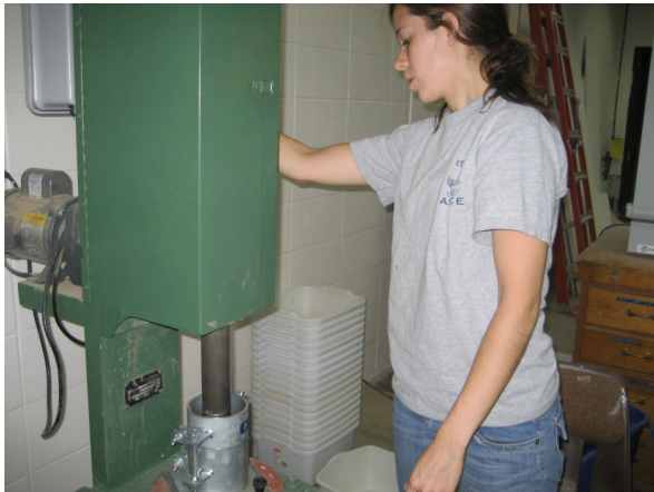
(79e) Compaction in a 4" split mold (79f) Planing the top after compaction
