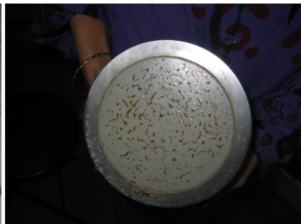
(27t) Moisture seen on the sensor base
