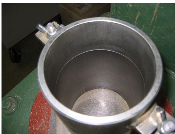
(27b) Mold cleaned and fitted to the compactor
