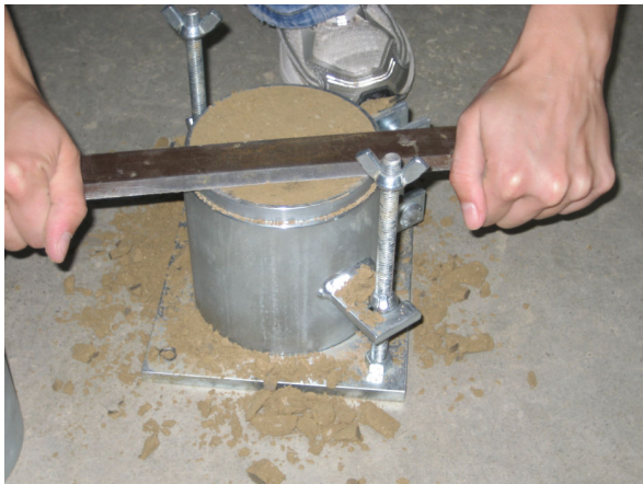
(79g) Planing the top of the sample (79h) Mold surface cleaned and dry density determined
