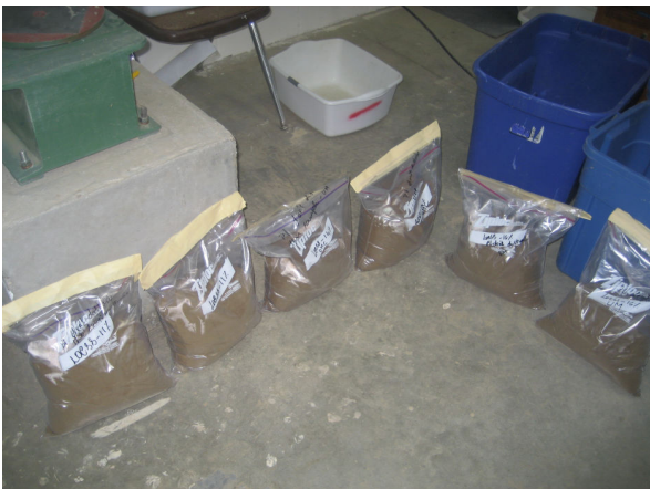
(79c, 79d) Samples packed in plastic bags after mixing required moisture and left for mellowing
