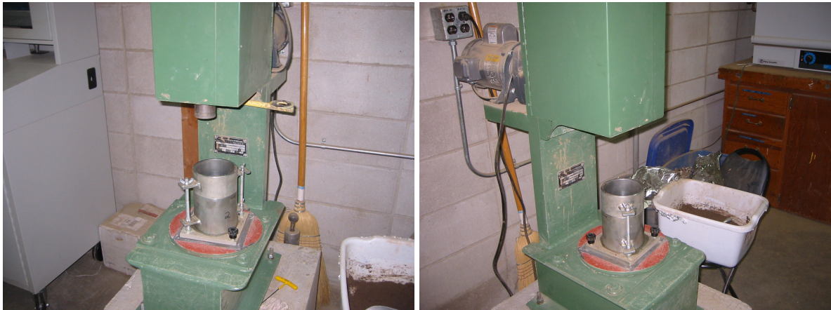
(27c,27d) Automatic Compactor set-up
